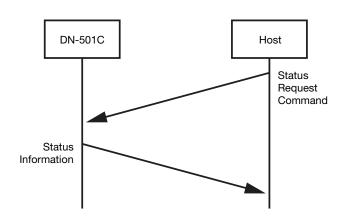
3. Status information automatically sent to the host when a change is made from DN-501C
